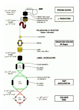
Figure 1: Schematic of a Muon Collider.
