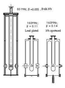
Fig. 3. Three different QWR's installed in the linac
