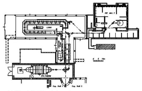
Fig. 1. Layout of the ALPI accelerator complex
