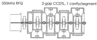
Fig. 9. Configuration of the match between the LEDA RFQ and the first section of the CCDTL.
