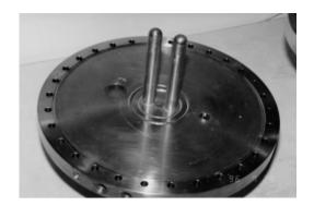
Fig. 4: End Flange and Rod Assembly.
