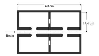
Fig. 3: Two Cell Separator Cavity.
