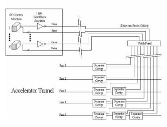
Fig. 2: RF Separator System.
