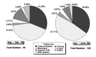
Fig. 2: Relative ratio of the linac operational faults.
