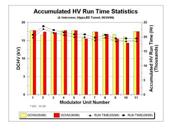
Fig.1: Accumulated run time of klystrons.
