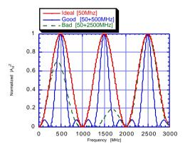
Fig. 3- Normalized square amplitude of spectrum envelopes vs frequency. The outer full line is the ideal one(only 500 MHz buckets evenly filled), the inner full line is a good one(mainly 500 MHz buckets filled. The dashed line is a bad one, with many 2500 MHz side buckets filled.
