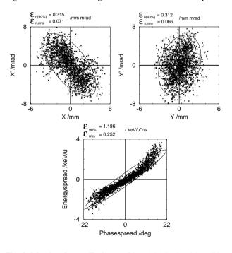
Fig. 3. Matcher Output Emittance Plots ( 16.5mA ; A/q=65 ).
