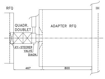
Fig. 1 Schematic of the Matching Section Components
