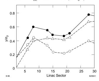
Fig. 1: Measured correlated and uncorrelated jitter development in the linac. While the correlated part (dash) shows the expected jitter profile (up and then down), the uncorrelated part (dash-dotted) grows steadily.
