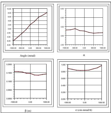
Figure 5. Steering, Twiss parameters vs. quadrant voltage unbalance
