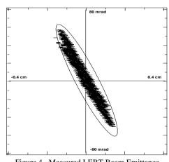
Figure 4. Measured LEBT Beam Emittance
