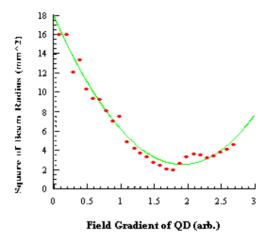
Figure 4 Relation of the square of the rms beam radius and the field of the quadrupole magnet (QD). The solid line shows a best fit curve.
