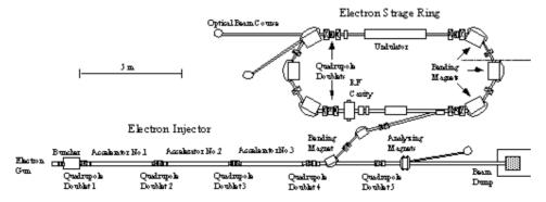
Figure 1 Layout of the electron accelerator.
