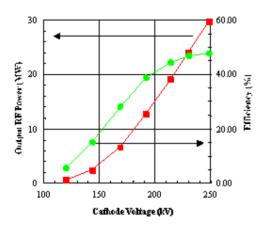
Figure 2 RF output power and the efficiency of the klystron (PV3030A2). The pulse width is 2usec.
