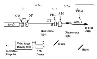
Figure 3 Schematic view of the beam monitor section downstream of the linac.
