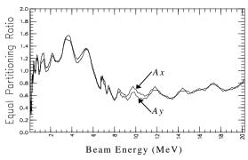
Figure 6. Shows the equipartitioning ratio (Ax and Ay) for the APT front end.
