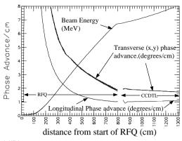
Figure 4. Zero-current phase advance per unit length in the RFQ and the CCDTL through the transition region. The transition from the RFQ to the CCDTL occurs at 800 cm.
