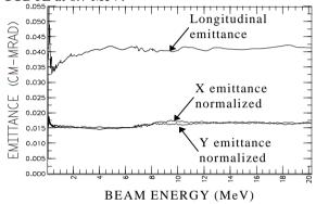
Figure 1. Longitudinal and transverse emittance versus energy. The transition from the RFQ to the CCDTL occurs at 6.7 MeV.
