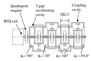
Figure 3. Following the RFQ, the accelerator consists of single-drift-tube CCDTL cavities of length  $3\beta\lambda/2$  spaced (nominally)  $5\beta\lambda/2$  apart. Quadrupole magnets are shown approximately centered in the spaces. Sideways-mounted coupling cavities maintain the proper phase between cavities.
