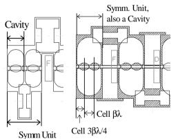
Figure 1. Cell, cavity, and symmetric unit in a 1- and 2-drift-tube CCDTL.
