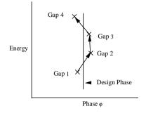
Figure 2. PARMILA adjusts the symmetric unit length and the entry phase until the design phase equals the average reference particle phase.
