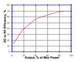
Fig. 4. Inductive Output Tube (IOT), Efficiency vs. Output Power
