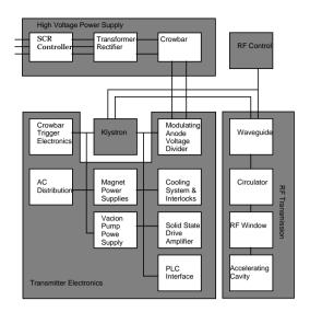
Fig. 2. RF system block diagram.
