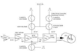
Fig. 1. Original 201 MHz Amplifier System.
