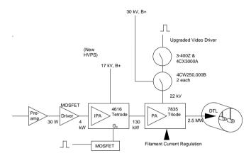
Fig. 2. 'Upgraded' 201 MHz Amplifier System.
