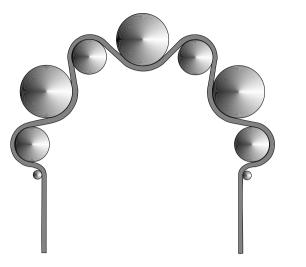
Fig. 2. Filament mandrel and filament. The figure shows how the tungsten wire is bent around the mandrel pegs to form the filament, as described in the text..
