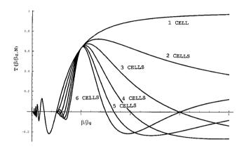
Fig. 1. Transit-time factor from the model versus  $\beta/\beta_G$ .
