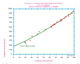
Fig. 3. Current measurements on the ESQ-Injector in excellent agreement with computer simulations.
