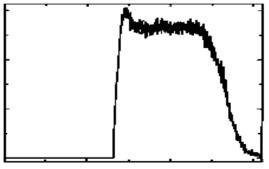
Figure 6: Current waveform at the end of the ESQ as calculated by WARP3d. Compare with Fig. 2. Horizontal scale at  $1\mu s$  per division.
