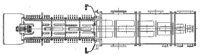
Fig. 1. The Injector System layout showing from left to right the source, the four-quadrupole ESQ accelerator, and the six-quadrupole matching section assemblies.
