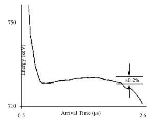
Fig. 4. Time profile of measured head-to-tail beam energy.
