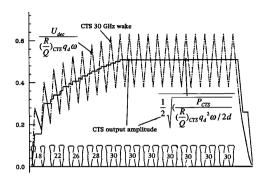
Fig. 2. Computer optimized bunchlet numbers, relative intensities, normalized 30 GHz CTS wake amplitudes (dashed, linear variations of ±23%) and the normalized CTS output amplitude.
