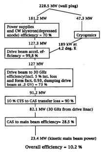
Fig. 6. Wall plug to main beam efficiency.
