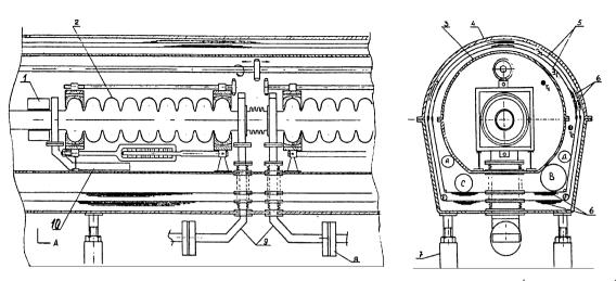
Fig. 1. 1 - quadrupole lens, 2 - accelerating cavity, 3 - helium vessel, 4 - cryo-module enclosure, 5 - heat  $(Y_2)$  and radiation  $(Y_1)$  screens enclosure, 6 - superisolation, 7 - supports, 8 - HF window, 9 - HF inputs system, 10 - load for high modes suppression, 11 - cavity adjusting mechanism, A, B, C, D, E, F - system of helium flow.
