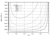
Figure 1: Attenuation constant corresponding to the fundamental mode of a coaxial waveguide versus the ratio of the radii of the inner and outer conductor *a* and *b*, respectively. The radius of the shielding serves as parameter.
