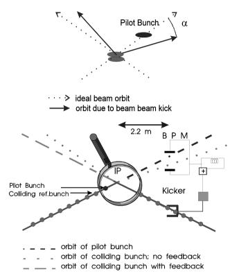
**Figure 1** Sketch of the interaction region layout and the location of the beam position monitor and the kicker magnet. The pilot bunch is the first bunch in the left train with no interacting counter part.
