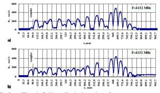
Fig.5. Electric field amplitude depends on frequency.
