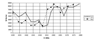
Fig.6. External Q-factor depends on frequency.
