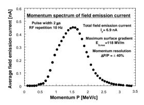
Fig. 7. Momentum distribution of the field emission current in the coupler cavity.
