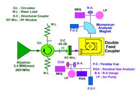
Fig. 4. Layout of the high gradient experiment.
