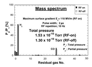
Fig. 8. Mass spectrum of the residual gases. There was no critical difference between rf-on case and rf-off case. No critical discharge occurred.
