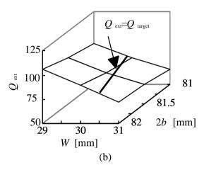
Fig. 3. (a)  $f_{res}(W,2b)$  and (b)  $Q_{ext}(W,2b)$ .
