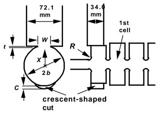
Fig. 1. Cross-sectional view of the coupler cavity (R=7mm and t=2mm).
