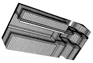
Fig. 2. MAFIA geometry for the Kyhl method simulation.
