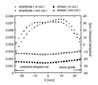
Fig. 7. Effect of the correction of an electromagnetic-field asymmetry by a crescent-shaped cut.
