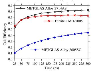
Fig. 3. Efficiency of the induction cell for converting the incident pulsed power into drive beam power as a function of pulse length for different core materials.
