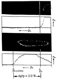
Fig. 2 Momentum Spectrum of the unaccelerated and IFEL accelerated electron Beam  $E_{l} = 40 \; MeV, \; B_{w} = 10 \; kG, \; \lambda_{w} = 2.9 - 3.1 \; cm, \; W_{l} = 1 \; GW.$
