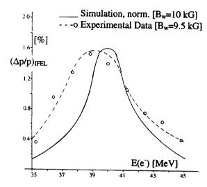
Fig. 3 Relative Energy Gain ΔE/E vs E, with B<sub>w</sub>, W<sub>1</sub> constant.
