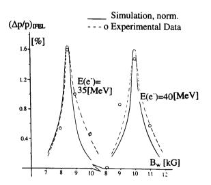
Fig. 4 Relative Energy Gain vs  $B_{\rm w}$  with E and  $W_{\rm l}$  constant.
