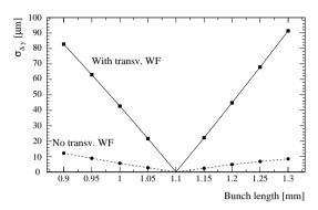
Figure 4: The rms trajectory change as a function of bunch length. A nominal bunch length of 1.1 mm is used as a reference for the other points. For this study we excited a 200  $\mu$ m rms trajectory oscillation in the SLAC linac. The solid line presents the full simulation, while transverse wakefields were switched off for the dashed curve.
