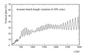
Figure 3: Vertical beam jitter in percentage of the expected beam size along the linac. The simulation assumes a random bunch length jitter of 10% and a bunch population of  $3.5 \times 10^{10}$ . The oscillations reflect a beta mismatch between the simulation and the design lattice.
