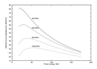
Figure 2: The effective shunt impedance of the BCDTL option for different operating frequencies.
