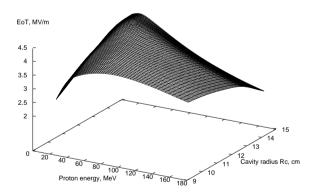
Figure 5: The  $E_0T$  surface for the BCDTL option.
