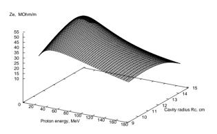
Figure 4: The  $Z_e$  surface for the BCDTL option.
