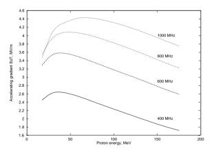
Figure 3: The accelerating gradient  $E_0T$  of the BCDTL option for different operating frequencies.
