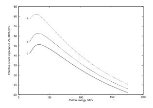
Figure 6: The effective shunt impedance for the BCDTL, a) -"ideal" structure, **b**- 6 cells tank without stems, c) 6 cells tank with stems  $r_s = 9$  mm.
