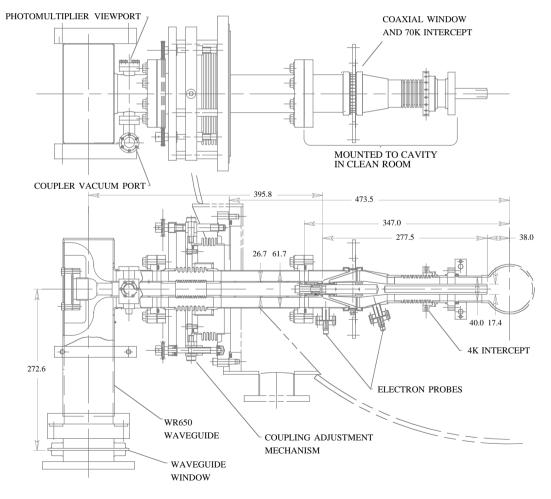
Figure 1. The Fermilab TESLA input coupler design.
