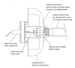
Figure 2. The design for the DC bias experiment.
