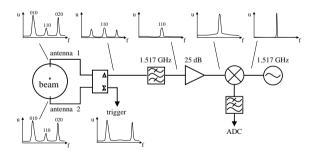
Figure 3: Signal processing scheme for a cavity BPM.
