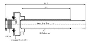
Figure 1: Cavity BPM with HOM absorber.
