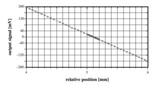
Figure 4: Measured linearity for the electronics.
