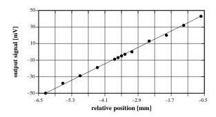
Figure 5: Test at CTF - output versus rel. position.
