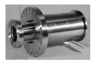
Figure 7: Stripline monitor, vacuum cover removed.
