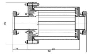
Figure 6: Design of the Stripline BPM.
