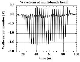
Fig. 5. Waveform of the multi-bunch beam.
