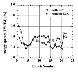
Fig. 4. Energy Spread of each bunch with and without ECS.
