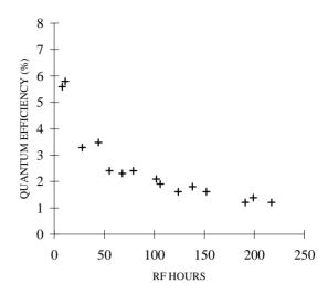
Fig.2 QE of Cs<sub>2</sub>Te photocathodes as a function of RF hours
