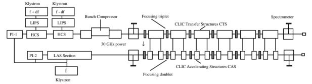
Fig.3 Schematic layout of CTF2
