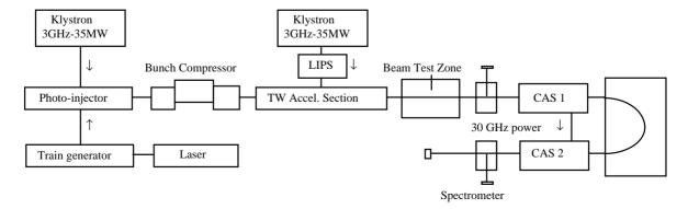
Fig.1 Schematic layout of CTF1
