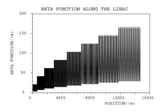
Figure 3: Scaling of the beta function along the linac. (Example: SBLC, a = 0.5).
