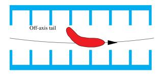
Figure 2: Wake field effects in the accelerator structures.
