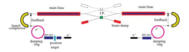
Figure 1: Linear Collider, schematic overview.
