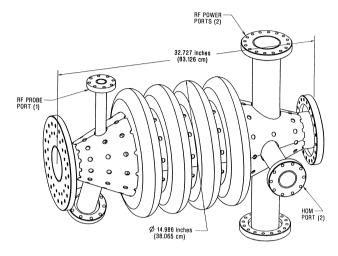
Fig. 6. Schematic of cavity design.
