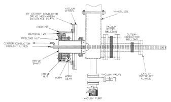
Fig. 3. Schematic of power coupler.
