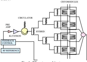
Fig. 4. RF system architecture.
