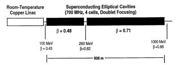
Fig. 1 Schematic layout of the APT SCRF linac
