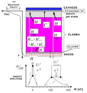
Figure 3: Production of H<sup>-</sup> at cathode and anode of the source and their energy spectrum.
