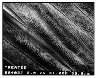
Figure 4: Excimer-treated polyester fiber showing surface roughening for improved look and feel [5].
