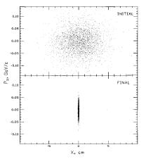
Figure 3. Transverse phase space  $(p_x-x)$  before and after a Li lens cooling channel which reduces  $\varepsilon_T$  from 0.01 to 0.00009 m-rad.
