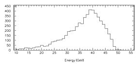
Figure 1: Bremsstrahlung energy distribution on luminosity monitor
