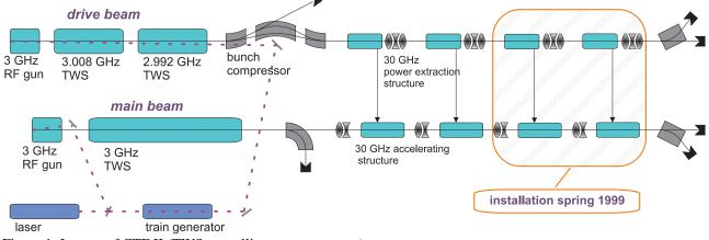
Figure 1: Layout of CTF II (TWS=travelling wave structure)
