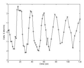
Figure 3: Wake potential measurement for a 15 GHz dielectric structure. Each data point is the change in the bend view centroid of the witness beam at the spectrometer 60° port.
