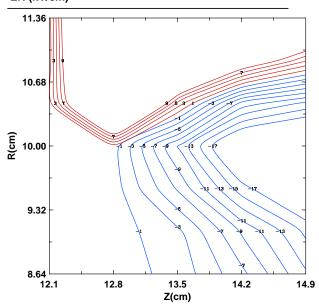
Figure 3: Contours of  $E_r$  near the outer radial boundary of the cathode. Between r=8.6 and r=10.0 cm the magnitude of this defocusing field nearly triples, leading to strongly nonlinear behavior in the electron beam's transverse phase space. Most of the nonlinearity occurs within  $1-2\ \Delta r$  of the beam edge.
