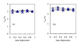
Figure 5: Ratio of the maximal radial extent to radius of matched beam vs  $\eta$  for mismatch parameter (a)  $\mu$ =0.6, (b)  $\mu$ =0.8, with different  $\sigma_0$ :  $\diamond$ -85°,  $\Delta$ -75°,  $\times$ -65°.
