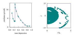
Figure 3: (a) Emittance growth of rms-matched Gaussian beams vs  $\eta$  and (b) phase-space distribution of rms-Gaussian beam at cell number=600 and  $\eta$ =0.245.
