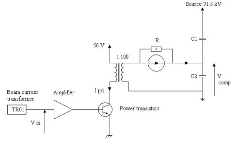
Figure 2: Block diagram of compensation scheme
