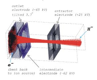
Figure 2: Ion Source Trajectories
