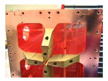
Figure 4: Cold Model End Detail, with Stabilizer
