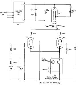
Figure 1: Basic Diagram of the Solid-State Deck
