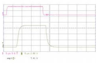
Figure 2: Klystron Current Pulse
