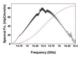
Figure 3: Spectral function for RDDS1 with all cells coupled and a perfectly matched HOM coupler. A systematic error in the fabrication is assumed to occur leading to a sinusoidal perturbation in the cell dimensions and the synchronous frequencies. The synchronous frequency perturbation has amplitude of 2 MHz.
