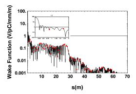
Figure 4: Wake function including the effects of a systematic fabrication error which results in a sinusiodal deviation in the synchronous frequency in the middle of the frequency band of the structure. Shown inset is the short-range wake in the range 0 to 2m.
