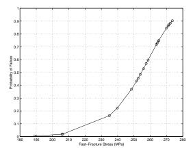
Figure 3: Probability of Failure in AL300 as a function of Stress State.
