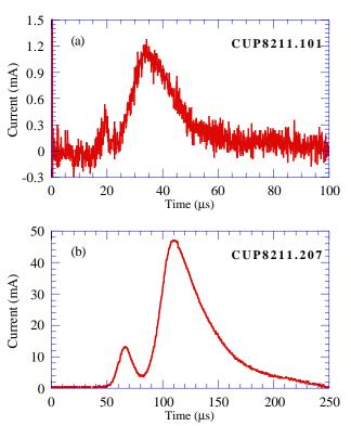
Figure 4. Typical output signals from the (a) back and (b) forward faraday cups. Beam interaction with the converter (1 mm thick Ta) occurred at time 0.
