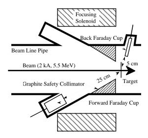
Figure 2. Schematic showing relative positions of the faraday cups with respect to the beam line and target.
