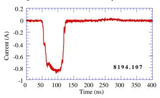
Figure 3. Typical output from the forward faraday cup.
