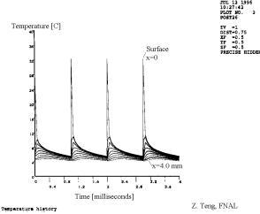
Figure 4: RF Pulse heating in the gun as a function of time.
