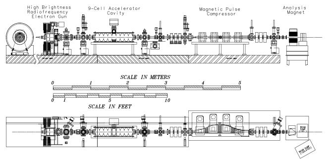
Figure 1: Layout of photoinjector components
