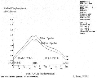
Figure 5: Outer wall radius change before and after rf pulse.
