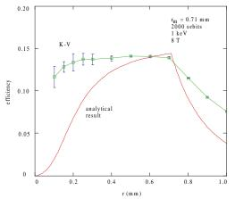
Figure 4: Comparison of numerical and analytical stripping efficiency models with electron beam radius.
